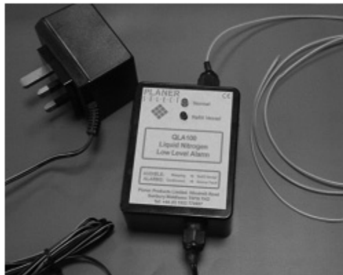
Figure 10 - A low-level sensor and monitor for generic LN 2 tanks. A built-in alarm system is triggered if the LN 2 level goes below the sensor position. Source: Planer plc. With permission.
