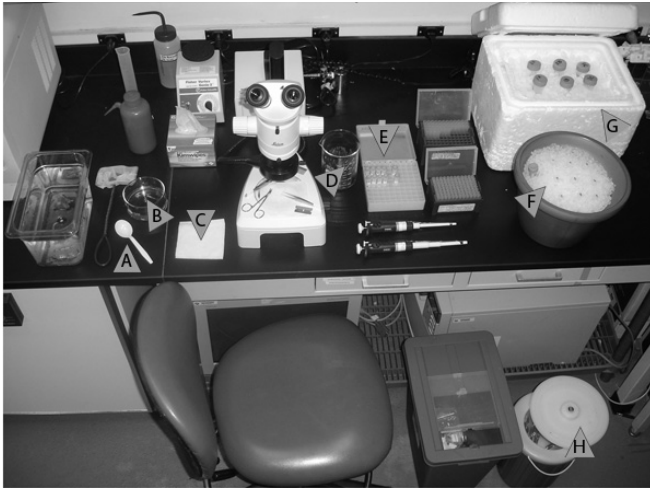
Figure 1 - Cryopreservation setup. Arrange reagents and equipment for efficient use during the protocol. Keep fish tank, net, tricaine on ‘wet’ side of the bench, while keeping the microscope and right side of the bench dry. A) Plastic spoon; B) Tricaine; C) Kim wipes to dry fish; D) Microfuge tube homogenizers; E) Labeled cryotubes; F) Chilled microfuge tubes with BSMIS; G) Chilled 50ml tubes on dry ice; H) Liquid nitrogen-containing Dewar.
