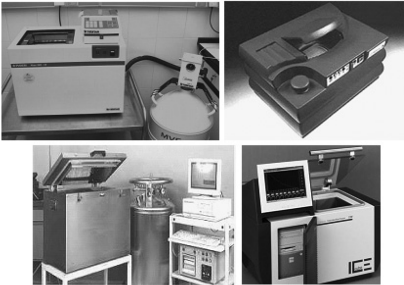
Figure 3 - LN 2 -based biofreezers: Kryo 560-16® (Planer plc; upper left), EF100® (Asymptote Ltd.; upper right), DigitCool 5300® (IMV Technologies; lower left) and IceCube 15M® (SY-LAB GmbH; lower right). Source: Dr. F. Martínez-Pastor (Kryo 560-16®) and the respective manufacturers. With permission.
