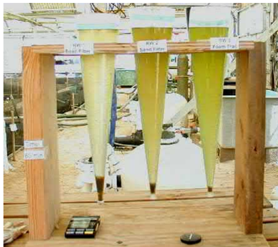
FIG. 7.2 One-liter Imhoff cones used to measure settleable solids.
