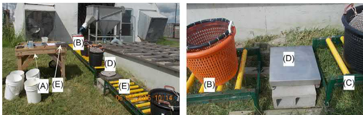
FIG. 8.18 Data recording station (A), preweighing conveyor (B) postweighing conveyor (C), and an electronic balance between the two conveyors (D) with remote display (E).
