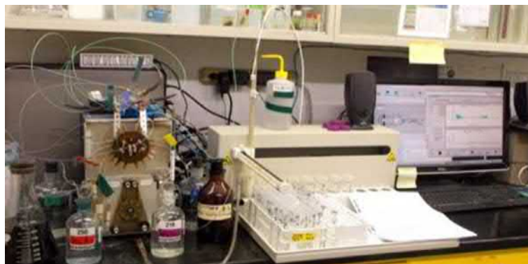
FIG. 5.21 Flow-injection analyzer used to measure ammonia, nitrite, nitrate, and phosphate at the Texas A&M-ARML.
