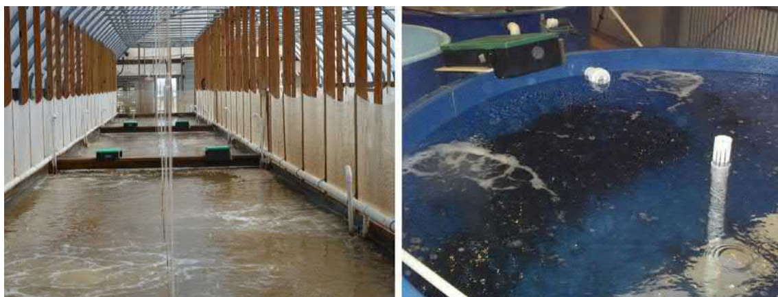
FIG. 5.19 Evenly spaced belt feeders mounted on walkways over a raceway, and a single belt feeder mounted on the side of a culture tank.
