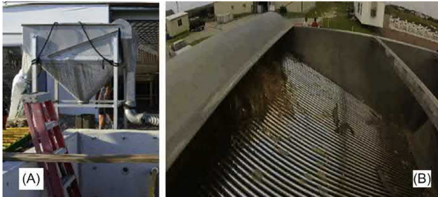
FIG. 8.21 Dewatering device (A) and close view of a dewatering rack (B) of a fish pump.
