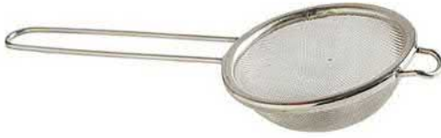
FIG. 8.12 Metal strainer for quantifying PL.
