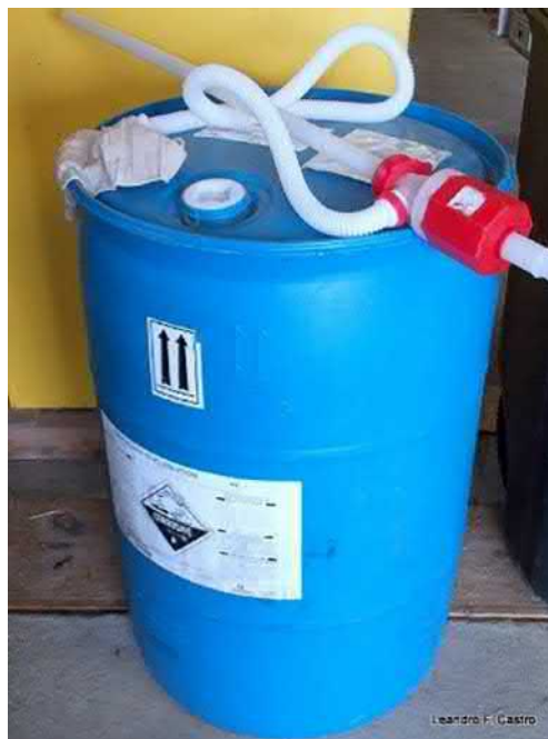
FIG. 6.4 Liquid (12.5%) sodium hypochlorite in a 200-L (55-gal.) drum with a siphon pump.
