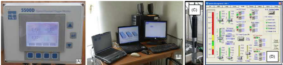
FIG. 5.29 YSI 5500D DO monitoring system: (A) on-site display, (B) computer display with audio, (C) optical probe, (D) programming and screenshot of alarm-setting software.
