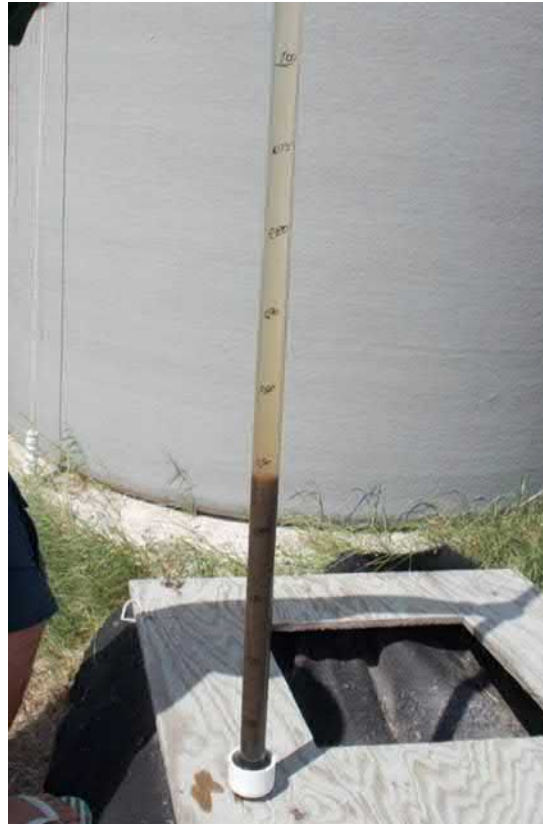
FIG. 11.1 Settled solids level from an anaerobic digester measured with a clear sampling tube.
