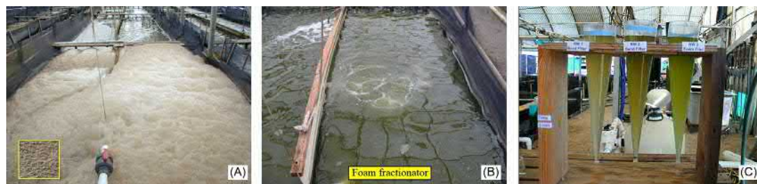
FIG. 14.3 (A) Heavy foam developed in the raceway with the pressurized sand filter, (B) a persistent algal bloom developed in the raceway with a foam fractionator during the 2003 nursery trial, (C) Imhoff cones, showing (left to right) water coloration in the raceways operated with bead filter, sand filter, and foam fractionator.
