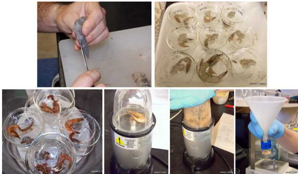
FIG. 7.4 Harvested shrimp being dissected, dried, and ground for ionic composition analysis.
