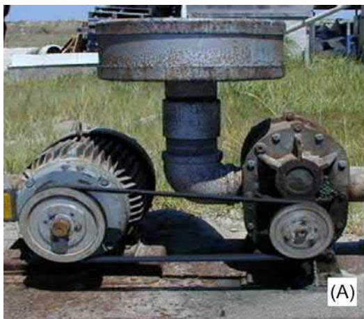
FIG. 5.6 Positive displacement blower with belt drive (A) and regenerative blowers (B) driving diffusers and airlifts in the Texas A&M-ARML 40 m 3 raceways. Blowers have inlet filters.
