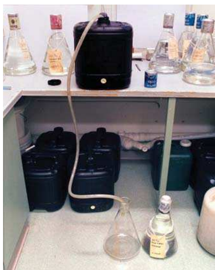
FIGURE 11.2. Seawater is collected and stored in 20-liter cubical black plastic containers. Seawater is siphoned into a 4-liter flask after adding 500-mL Milli-Q water.
