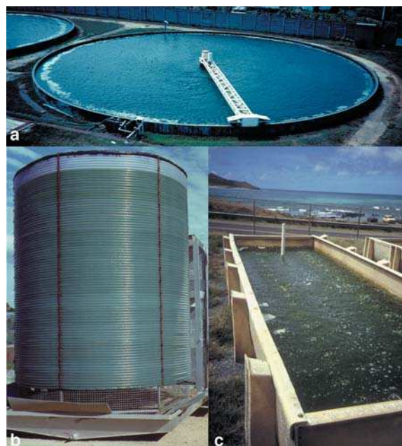
FIGURE 14.2. (a) Center-pivot pond used for the cultivation of Chlorella in Taiwan. Note the variable mixing effectiveness, as illustrated by the foaming at the pond perimeter. (b) Biocoil, a 1,000-liter helical tubular photobioreactor. (c) Deep aerated tank used for the culture of Nannochloropsis for aquaculture.
