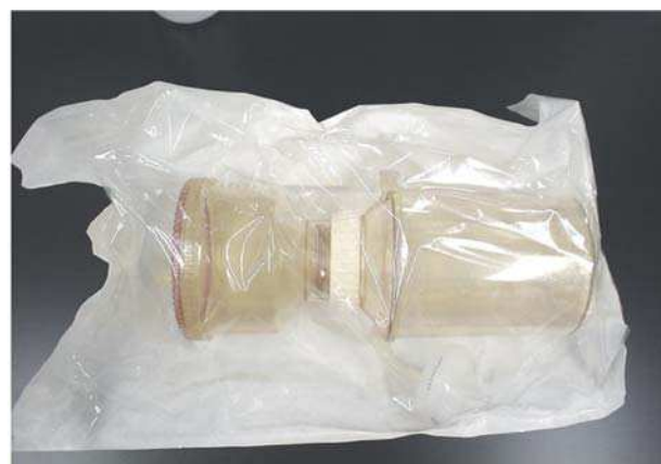
FIGURE 5.7. A reusable filtration apparatus inside an autoclavable bag.
