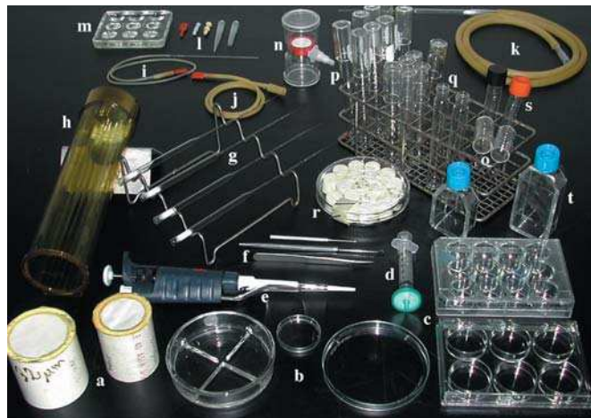
FIGURE 6.1. Assortment of isolation supplies. (a) Screens for removing larger animals and algae; prepared from PVC pipe and Nitex netting. (b) Glass and plastic dishes. (c) Multiwell plates. (d) Syringe with 0.2- \mu m filter. (e) Pipetteman. (f) Small loop, fine metal probe, and forceps. (g) Pasteur pipettes, with tips drawn to produce micropipettes, arranged on a metal rack. (h) Sterile Pasteur pipettes in plastic can, resting on a simple metal support to keep the opening off the table surface. (i) Glass capillary tube, small tubing, and red mouthpiece. (j) Isolation mouthpiece (red), small tubing connected to final short piece of large tubing that forms a tight seal when a Pasteur pipette is attached. (k) Large isolation tubing with plastic pipette tips at both ends, one serving as a mouthpiece and the other supporting a Pasteur micropipette. (l) Commercial mouthpieces (red, white, yellow) and two plastic pipette tips (right one with pointed tip removed), which can be used as mouthpieces. (m) Glass spot plate that can be used to rinse cells during isolation. (n) Small sterile filter apparatus. (o) Glass slip caps that cover either smooth or threaded test tubes. (p) Smooth, unthreaded test tubes covered with slip caps. (q) Threaded test tubes covered with slip caps. (r) Sterilized test tube caps that can replace slip caps or be used when a culture tube cap is dropped or contaminated. (s) Plastic threaded test tubes (black cap, orange cap), which are sterilized by the manufacturer. (t) Two blue-capped tissue culture flasks, sterilized by the manufacturer.
