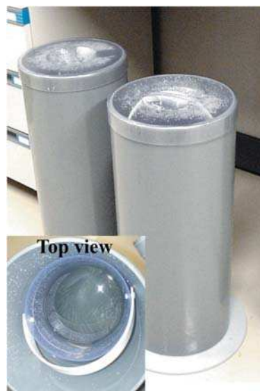
FIGURE 5.3. Detergent baths for cleaning glass inoculation pipettes (inset: top view of bath).
