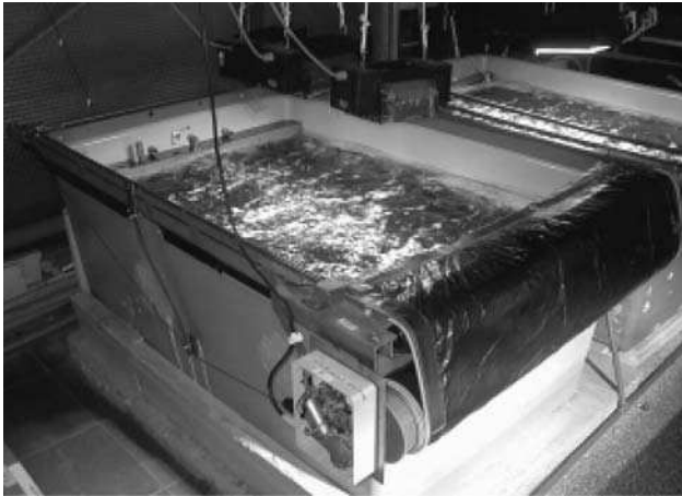
FIGURE 21.9. A 2,000-liter tank with automatic blind consisting of a light-tight plastic cover on a motor-driven roll.
