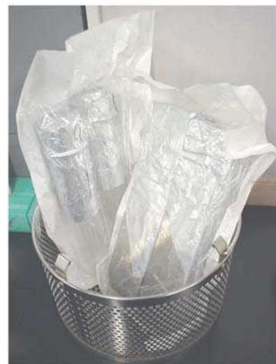
FIGURE 5.9. A stainless steel basket for holding items in an autoclave. The basket contains Pasteur pipette canisters covered with autoclavable bags. Note that the cap junction of a pipette canister is covered by aluminum foil.
